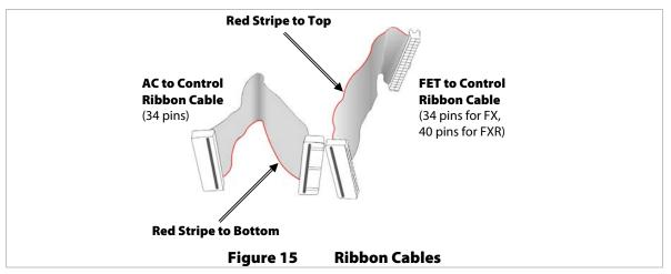
Install the ribbon cable that is bent on one end to the FET PCBA and the Control PCBA. (See Figure 16 and also Figure 7 if necessary.) In the FX inverter, this cable has 34 pins. In the FXR inverter, it has 40 pins. Make sure the red stripe is oriented toward the **top** of the chassis. Push down on each end until the levers click and the plug is secure.
